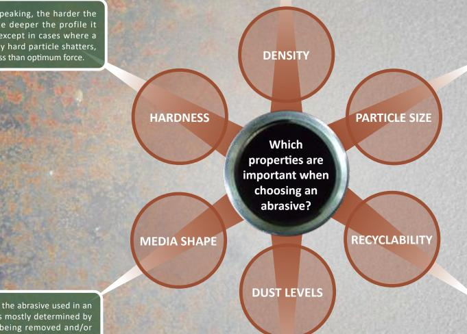
All things being equal, the bigger the particle, the deeper the indentation it will make, but blasting large particles will result in fewer impacts than an equal volume of smaller particles. Small particles clean faster, provide better coverage, and result in a more uniform profile. The most efficient approach is to use the smallest particle necessary to achieve the desired profile.
